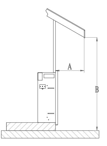
The overhang (A) must extend at least 1/2 the roof-line height. Height is measured from the base of the fireplace. For example: if the roof-line (B) is 8' above the base of the fireplace, the overhang (A) must be at least 4'.
