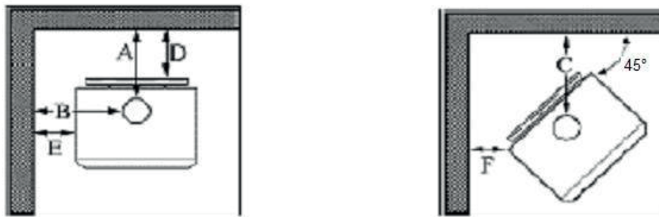
Figure 4. a) Parallel installation, b) Corner installation
