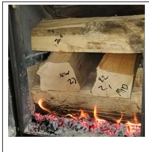
Run 2 – Test Fuel Loaded into Stove
