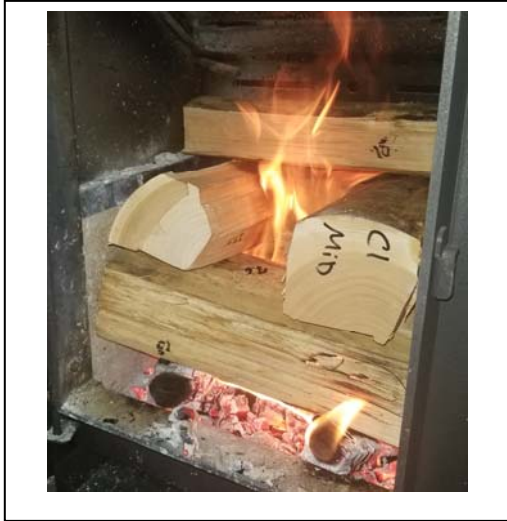
Run 1 – Test Fuel Load In Stove
