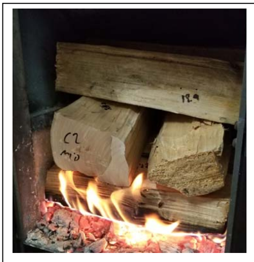
Run 4 – Test Fuel Loaded into Stove
