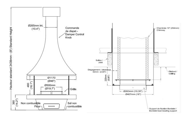
Warning: For centrally-located fireplaces, a minimum clearance to combustibles of 1.2m (48") must be maintained 360 ° around the fireplace. For single wall smoke pipe, a minimum 45cm (18") clearance to combustibles must be maintained and, when connected to the Bordelet Load Bearing Support, a minimum 220mm (8- 11/16") clearance from the top of smoke pipe mounting flange to the ceiling must be maintained, especially with slanted ceilings. Adjust the height of the Load Bearing Support accordingly.
