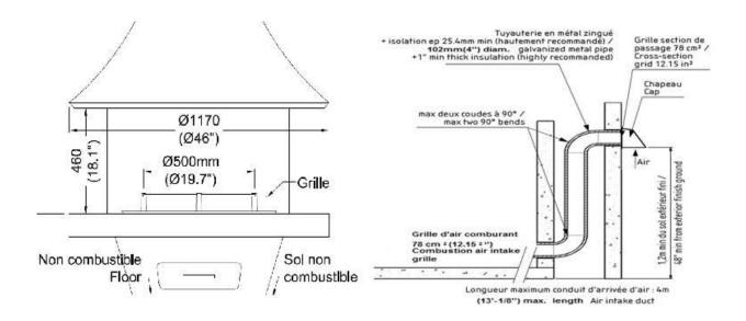
Caution: the Outdoor Combustion Air intake must not come from an attic, garage, carport, basement, the chimney's enclosure or be less than 3m (10') from a gas meter, a fuel/propane tank or any other device that may emit fumes or gases, such as the exhaust of a motor vehicle.
