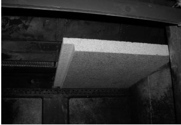
Figure 16 (cont.) - Removing/Replacing the Baffle for Inspection
