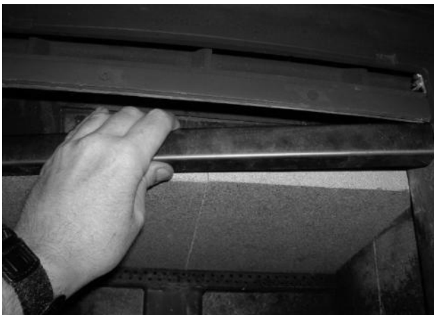
Figure 16 - Removing/Replacing the Baffle for Inspection
