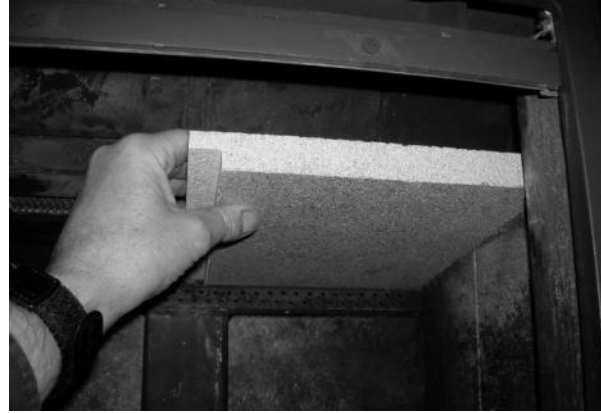
Figure 16 (cont.) - Removing/Replacing the Baffle for Inspection
