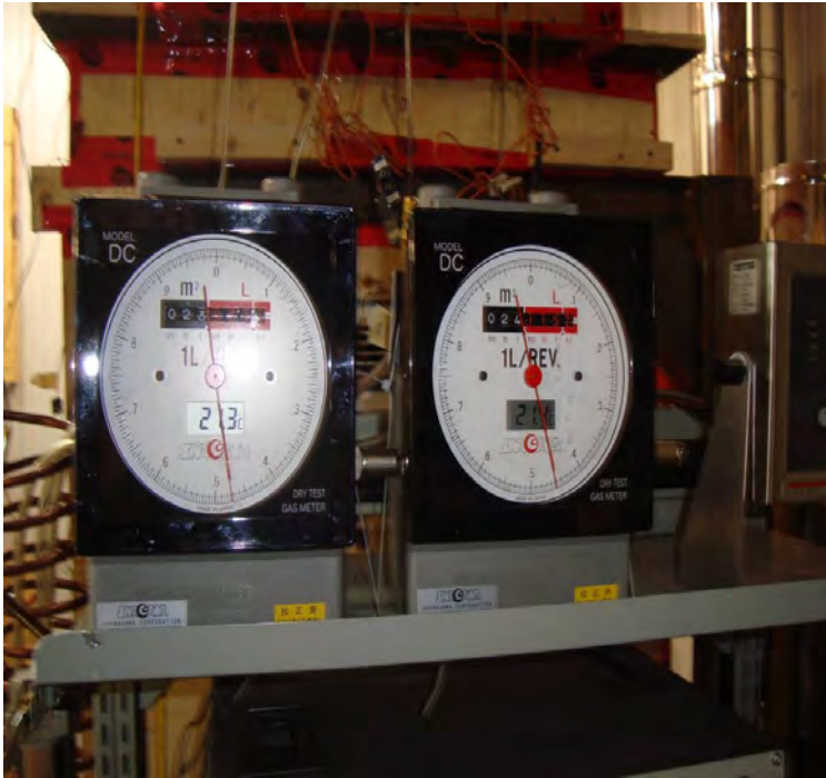
Picture 11: Dry gas meter
