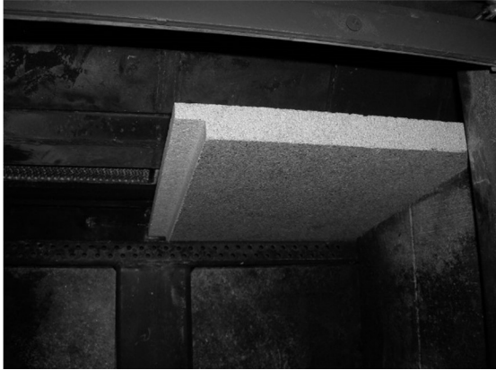
Figure 186 (cont.) - Removing/Replacing the Baffle for Inspection
