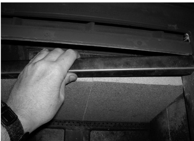
Figure 16 - Removing/Replacing the Baffle for Inspection
